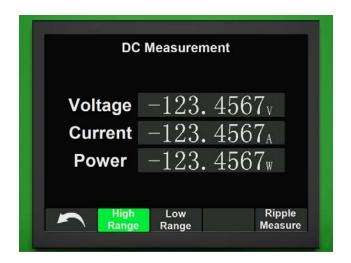
After clicking "Ripple Measurement", this instrument enters the ripple measurement function mode as shown below, and the magnitude of the voltage and current and the ripple effective value will show.
